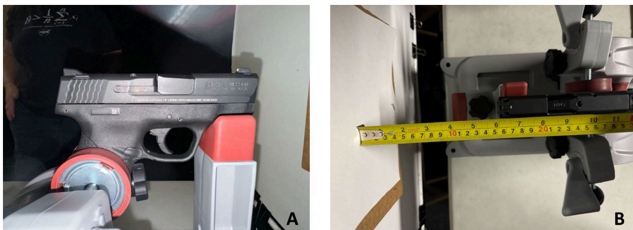
Figure 1. (a) Shooting vise setting using the Smith & Wesson M&P9 Shield, caliber 9 mm Luger, semi-automatic pistol used to obtain all samples. (b) Demonstration of measurement from the muzzle of the firearm to the center of the target material at 6 inches. The same set was applied for all distances tested.
